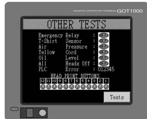
For example, if you disconnect the Yellow Cycle Interruption cords, the indicator to the right of Yellow Cord displays an **OFF** indication.
