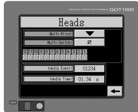
To select print stations for 2-9 print strokes, press the button to the right of **Multi-Switch** until the button displays **2-9**.
