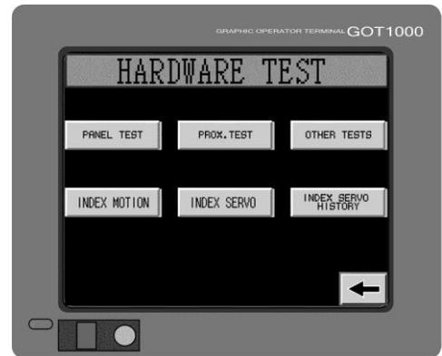
The **PROX. TEST** screen provides a visual indication of all the proximity switches used to control the index and print heads. The indication is used to confirm the operation of the particular proximity switch.
