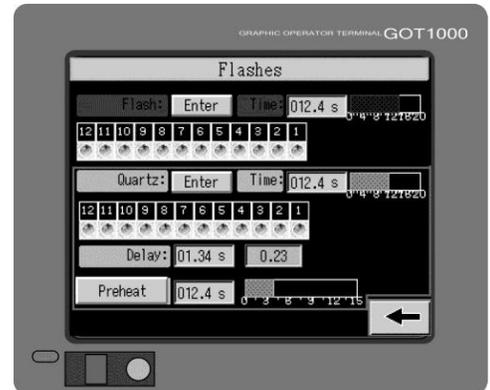
Press the print station number to operate as a quartz flash cure station. After you press the print station number the indication changes to green and displays a vertical line for **On**. If you press the print station number again, the indication changes back to red and displays a zero for **Off**.
