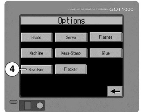
The button (5) to the right of **Revolver Mode** displays either **On** or **Off**. To change between **On** and **Off** mode press the button. Press the button until **On** displays to program or operate in the **Revolver Mode**.
