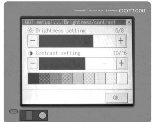
A graduated scale is displayed at the bottom of the screen and may also be used to set the brightness and contrast of the display screen. Press the shaded cell in the graduated scale which most approximates the brightness and contrast setting you require. When you are finished, press the **OK** button.
