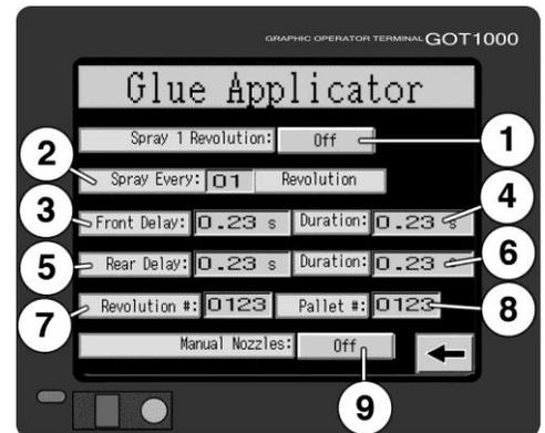
right of **Spray Every**; a numeric keypad is displayed. Enter the number from 1 to 99 and then press **Enter**. Your selection for **Spray Every** is now displayed in the data entry cell.
