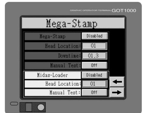
**Mega-Stamp Down Time** **Down Time** is used to select the amount of time that the **Mega-Stamp** heat platen is down in contact with the foil and garment. To adjust the **Down Time**, press the data entry cell to the right; a numeric keypad is displayed. Enter the down time and then press **Enter**. Your selection for the **Down Time** is displayed in the data entry cell.
