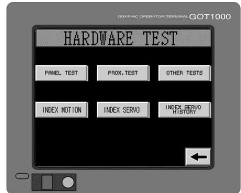
**Panel Test** The **PANEL TEST** screen provides a visual indication of all the switches used on the main control panel. The indications confirm the correct operation and position of the particular switch or push button.
