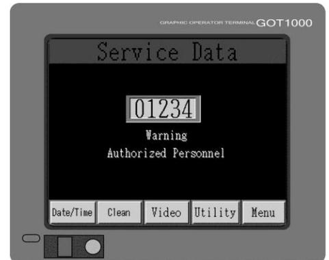
When you are finished cleaning the screen surface, press the top corner buttons simultaneously. This will return you to the **Service Data** screen.
